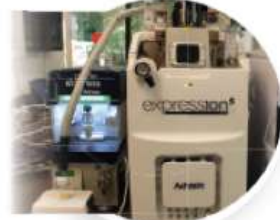
Inert atmospheric solids analysis probe (IASAP)
