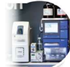
Online Flash/CMS - mass directed fraction collection
