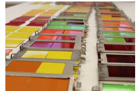
Coating testing/Anti corrosion
